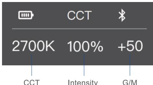
2.1.1 CCT adjustment: Hit the FN button to select the CCT. Press the +/- button to adjust the CCT in at least 100K increments from 2700K to 8500K.
