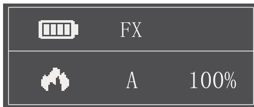
2.2.1 Hit the FN button to select the Effect/Speed/Intensity. Press the +/- button to adjust the settings.
